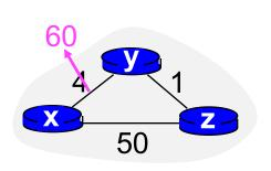
$$\begin{array}{l} D_{y}(x) = \min\{c(y,x) + D_{x}(x), c(y,z) + D_{z}(x)\} \\ = \min\{60 + 0, 1 + 5\} = 6 \\ & \longrightarrow \text{Routing Loop} \\ D_{z}(x) = \min\{c(z,x) + D_{x}(x), c(z,y) + D_{y}(x)\} \\ = \min\{50 + 0, 1 + 6\} = 7 \\ & \longrightarrow \text{Count-to-infinity} \end{array}$$
