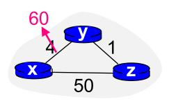
$$\frac{D_{y}(x) = \min\{c(y,x) + D_{x}(x), c(y,z) + D_{z}(x)\}}{= \min\{60 + 0, 1 + \infty\} = 60}$$
